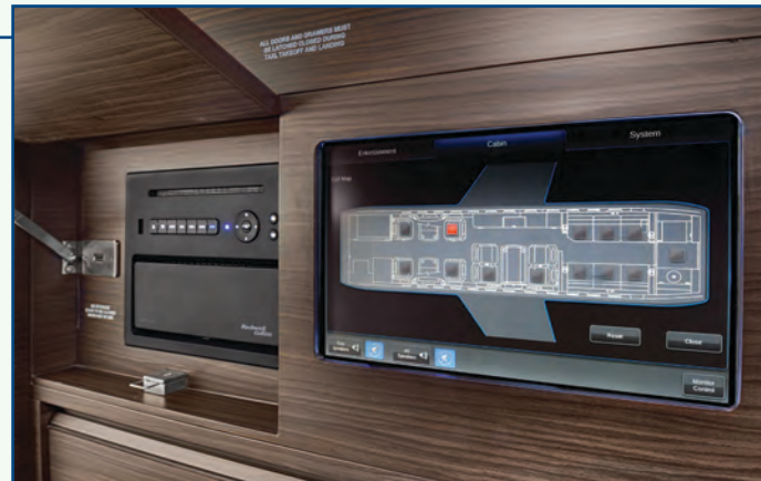
A nine inch touch screen provides full system control including galley functions, cabin lighting, entertainment, temperature and cabin call.
