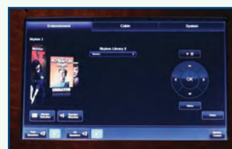
A nine inch touch screen provides full system control including galley functions, cabin lighting, entertainment, temperature and cabin call.
