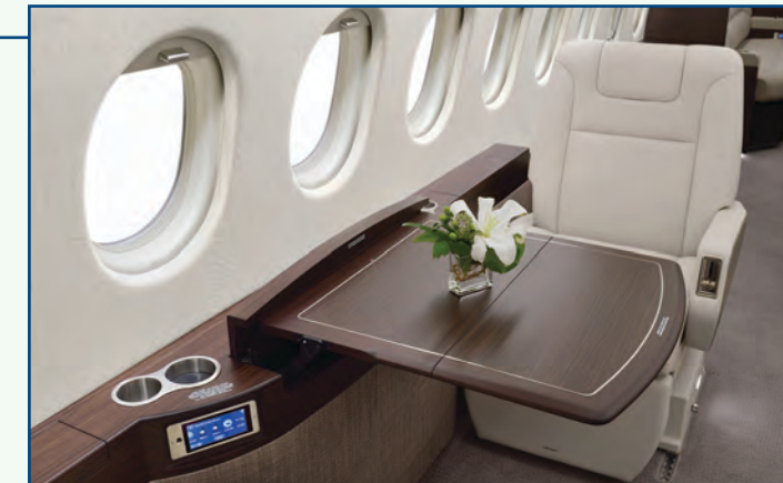
Passenger control units are installed at every cabin seating position and are layered similar to an iPhone.
