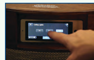
A nine inch touch screen provides full system control including galley functions, cabin lighting, entertainment, temperature and cabin call.
