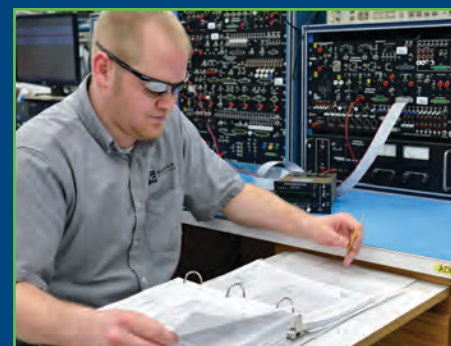
Patrick Klein, avionics tech, is running a TH250 Tac/Com control head through a function test. This unit provides tactical channeling for up to four independent transceiver systems.
